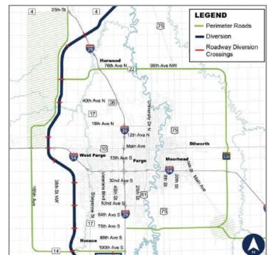
Figure 1.7 Potential Perimeter Roadway Alignments
