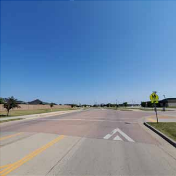
Raised, stamped, and stained intersection near Freedom Elementary in West Fargo, ND
