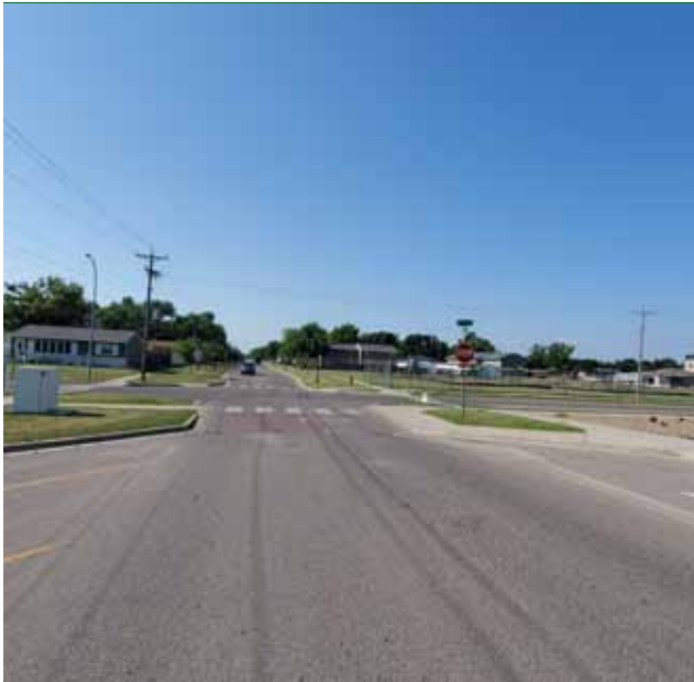
Curb extension narrows crossing of 1 st St E near South Elementary School in West Fargo, ND
