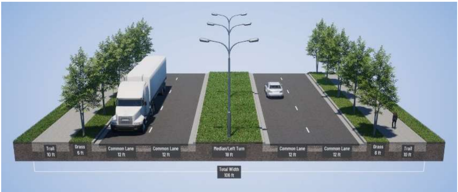
Figure 3.5 – Commercial Arterial Typical Section
