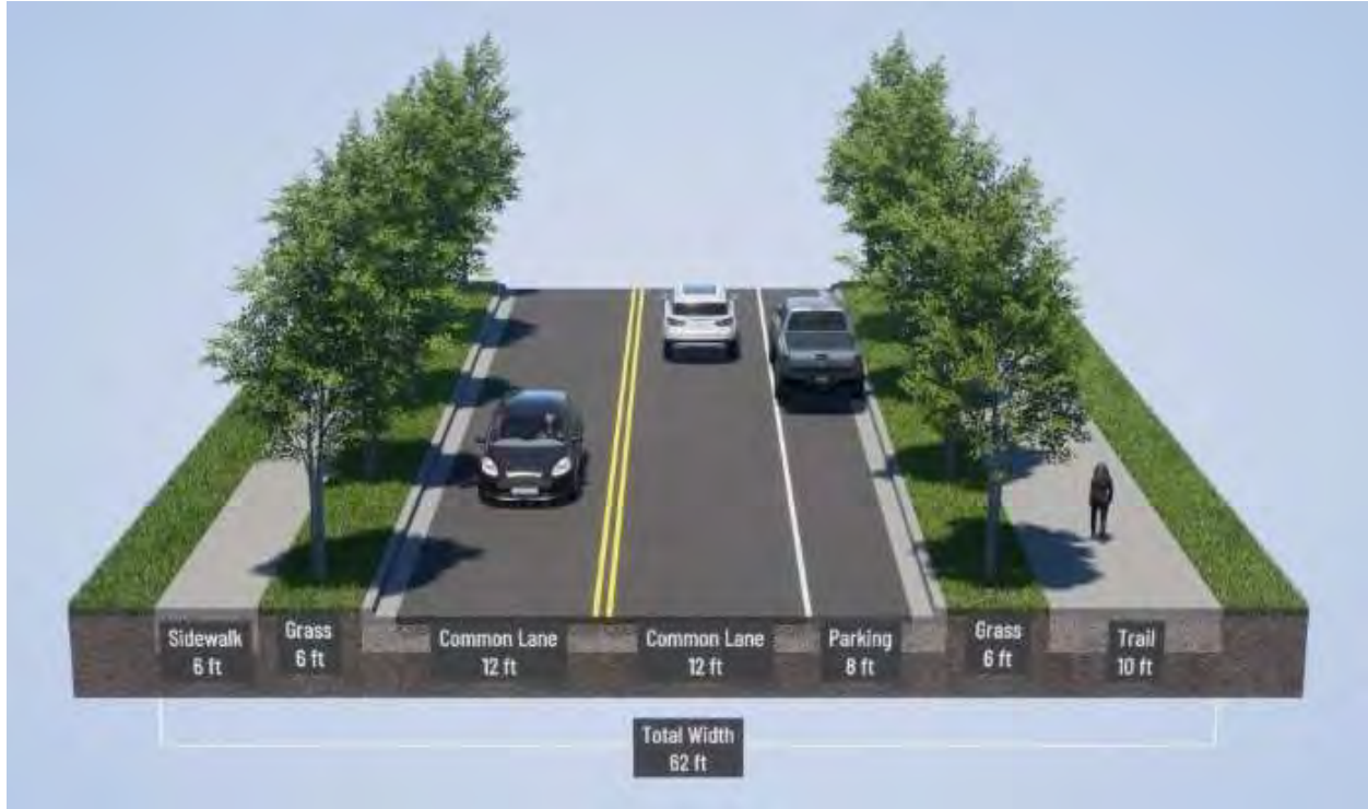
Figure 3.11 – Shared Use: On-Street Parking
