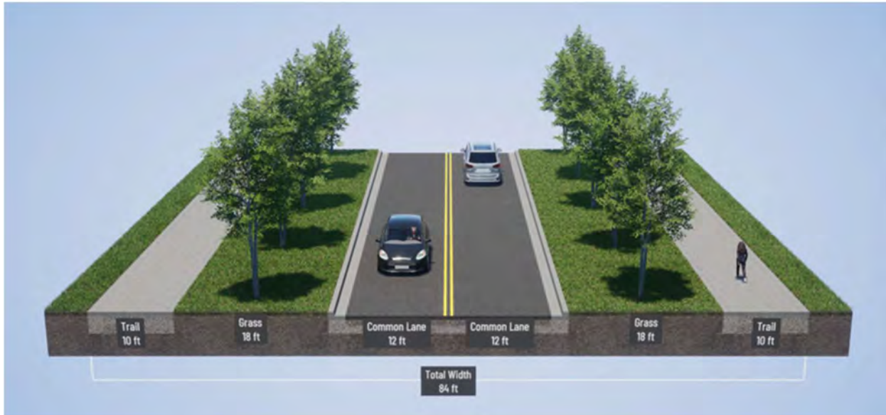
Figure 3.7 - Mixed Use Arterial Typical Section, Extended Boulevard
