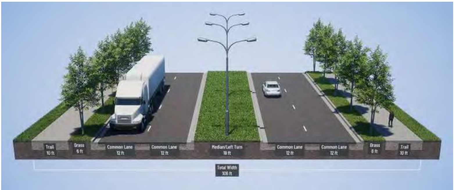
Figure 3.5 – Commercial Arterial Typical Section
