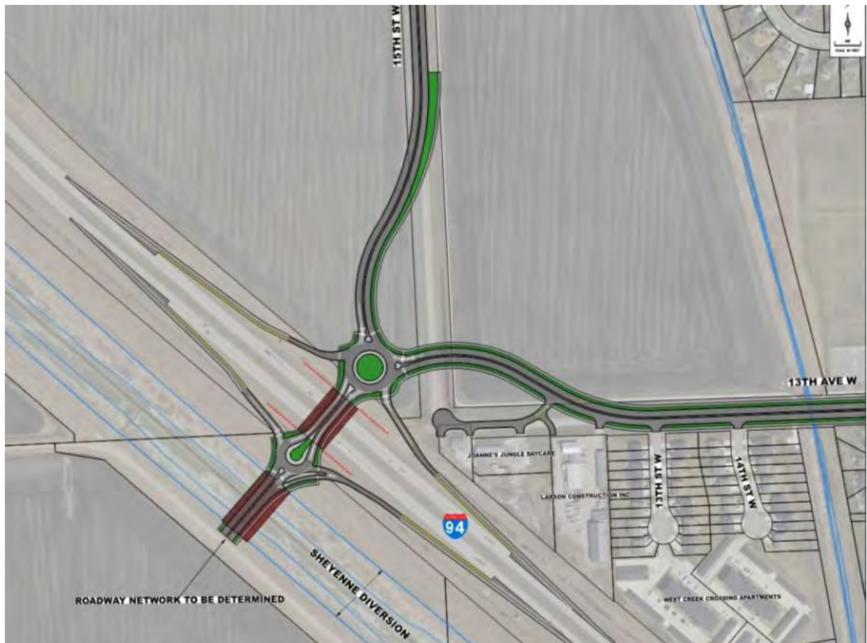
Figure 4.11 – 15 th Street and 13 th Avenue Roundabout Interchange
