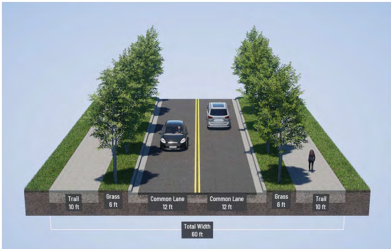
Figure 3.6 - Mixed Use Arterial Typical Section
