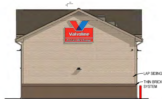
4 EXTERIOR ELEVATION (NORTH) Scale: 1/8" = 1'-0"
