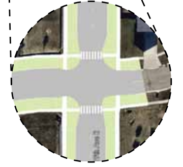
Curb Extensions and Crossing Improvements @ 19th Ave E
