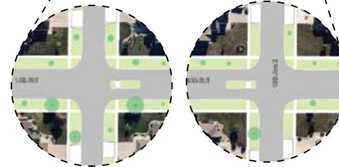
Median Refuge Islands - 1700 Block
