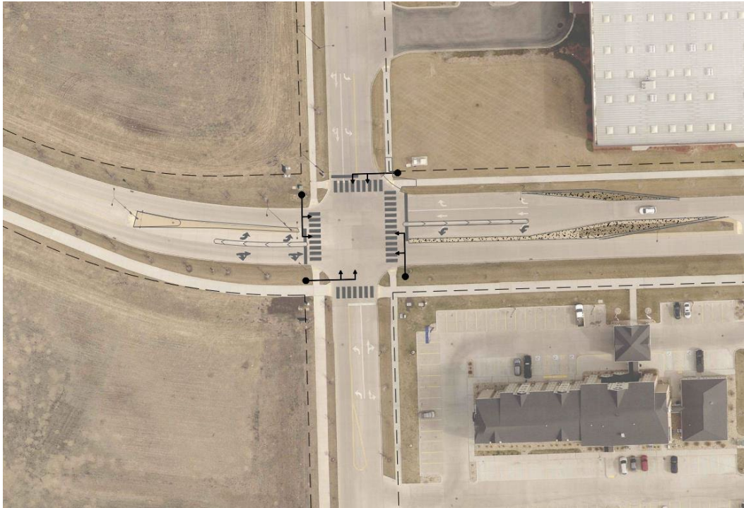
Traffic Signal with Neutral Left and Extended Turn Lanes Conceptual Layout:
