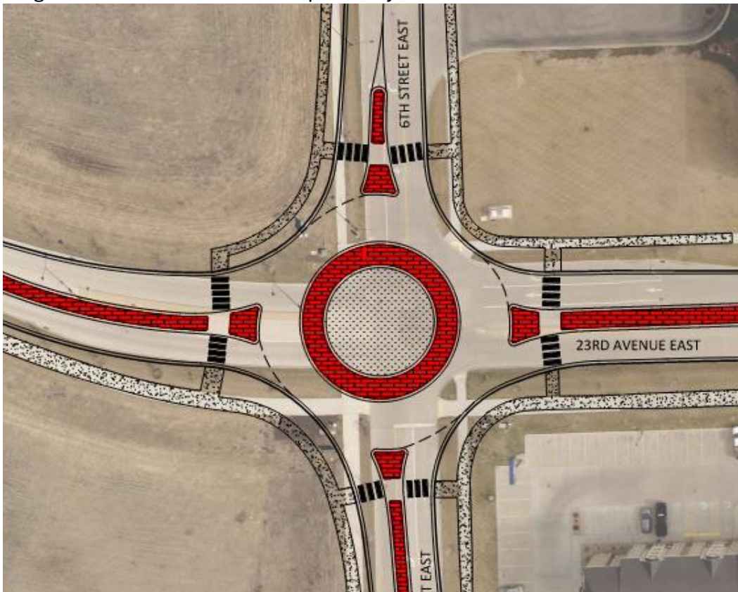
Single Lane Roundabout Conceptual Layout:
