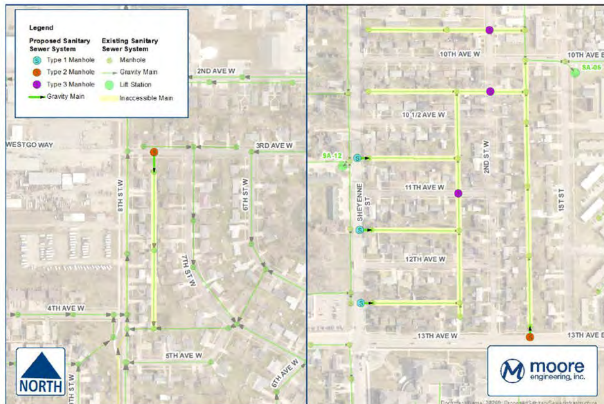
Figure 1 – Manhole Location – Dawns Addition
